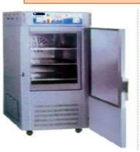
•Temp. Controlled by Digital Temp. controller. Inner Chamber double walled Stainless Steel Outer Body M.S. Duly epoxy powder coated/Stainless Steel. •Stainless steel with perforated adjustable shelves.
