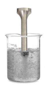
Choosing the appropriate horn is extremely important. The sample volume to be processed is directly related to the tip diameter. Smaller tip diameters (Microtip probes) deliver high-intensity sonication, but the energy is focused within a small, concentrated area. Larger tip diameters can process larger volumes but offer lower intensity.
