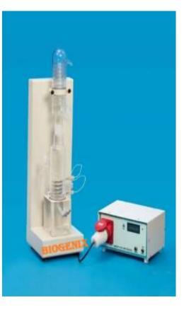
4) **Reservoir Level Sensor** – is provided for automatic operation of the unit. When the reservoir is full with distilled water the unit switches off, the unit switches on when distilled water is drawn from the reservoir
