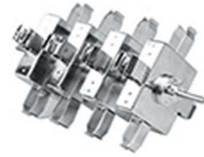
Cat. No.: 18900147 For 16*50ml centrifuge tube Held vertically
