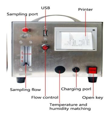
BioGenix Particle counter back side facility with sampling port, USB, Printing facility, sampling flow, flow control, charging port, Temperature and humidity matching, and open key.
